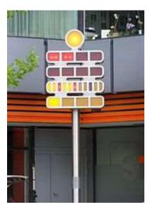
The Mengenlehreuhr consists of 24 lights which are divided into one circular blinking yellow light on top to denote the seconds, two top rows denoting the hours and two bottom rows denoting the minutes.
